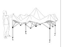
Remove the ceiling canopy and place the ceiling canopy on top of the rack. Grab the middle part of the frame and pull it outward until the frame is fully
