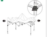
Hold down the latch, grab the rack, lift it up until it's fullylocked, and then the rack is fully unrolled, velcro on the foursides of the interior holds the ceiling cloth to the shelves.
