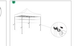
Notice, that there are three Hole location on the shelf, representing different heights. You can change gears by pulling the circular pull ring at the bottom of the shelf.
